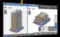
■ Zlider Bar allows you to vertically cut out building model elements for best map visualisation
